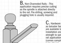
C. Hardware such as baluster fasteners are available to ease installation and add strength to spindle/ rail application. (comes complete with instructions)
